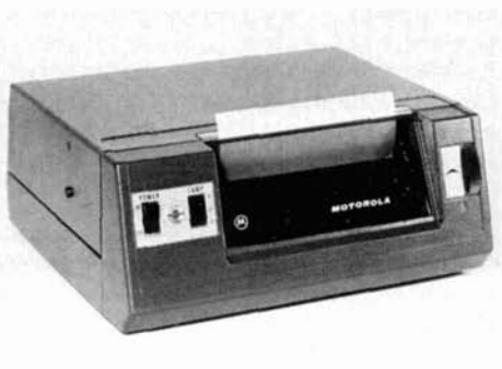
The Motorola VP-100 miniaturized teleprinter. It uses a special code for communications security and features selective calling.
